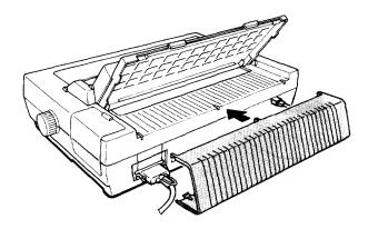
Note: The cable cover should always be attached when you use the printer.
